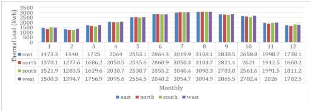
Figure 9: Shows the thermal loads of residential villas during the months of the year in the four main orientations (Devised by the Researchers).
