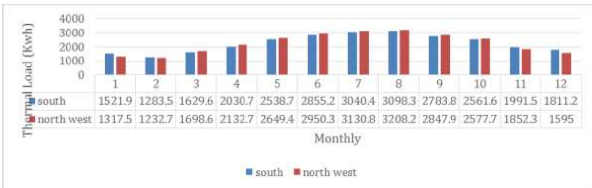
Figure 8: Shows the difference in thermal loads between the current orientations of residential villas (Devised by the Researchers).
