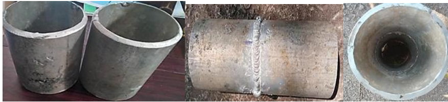
Fig. 1: A6063 T5 aluminum alloy welded pipe.
