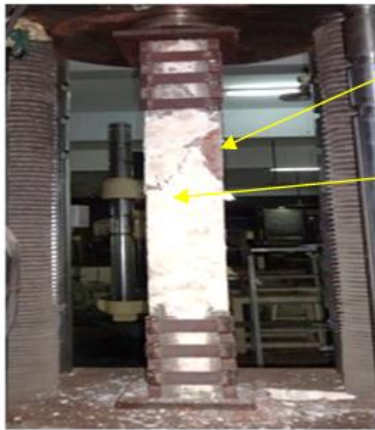
Figure 6 Failure mechanism of the partially end strengthened RC column NS1.
