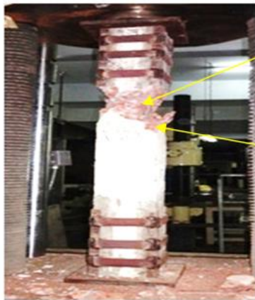
Figure 8 Failure mechanism of the Partially end strengthened preloaded RC column NS2.
