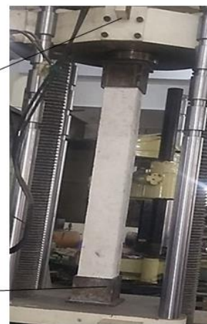
Figure 3: Preloading test set up using steel heads at Top and Bottom of the Specimen.
